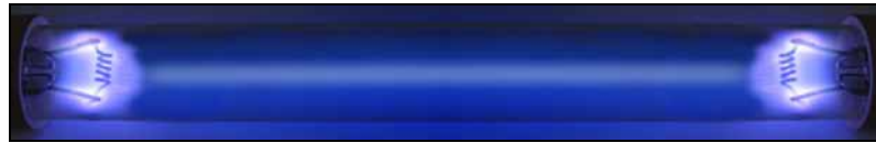
The Filaments and Arc in a UV Lamp
