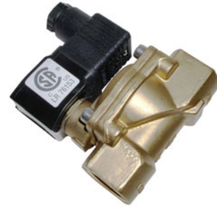
A solenoid valve shuts off the flow of water, if the intensity of the UV lamp goes down
